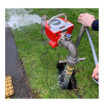
By using the "TSI Digital Flowmaster 250", the latest digital flow testing equipment available, our engineers are able to digitally record a fire hydrants water pressure and the flow rate reading to a 98% accuracy.
