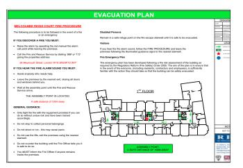
The **fire equipment plans** detail the location of the installed fire detection and alarm system assets, as-well as firefighting equipment.
