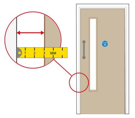
More than 230 (34%) fire doors inspected had excessive gaps between the door and its frame (i.e. over 3mm)
