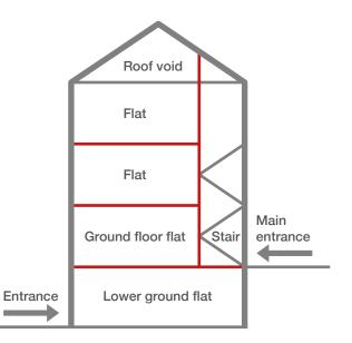
Fire-resisting compartment wall and floor
